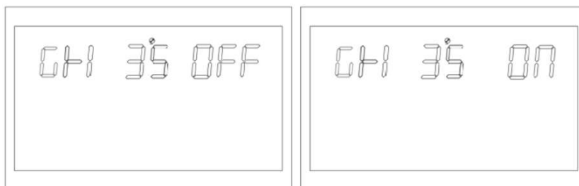
Figure 1-43 Grid-connected inverter function setting page
