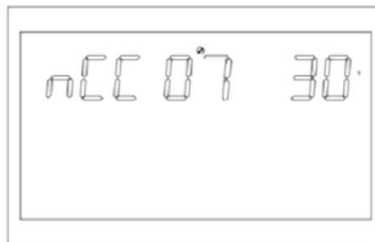
Figure 1-18 Setting the maximum charging current
